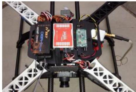
Fig4 Flight Controller
