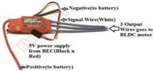
Fig2 Electronic Speed Controller
